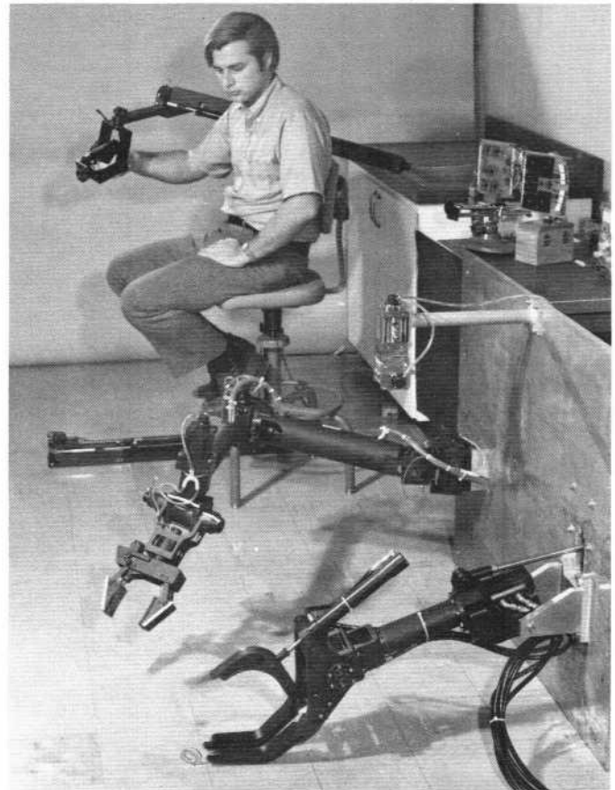
Fig. 7. The RUWS manipulator suit during laboratory testing.
